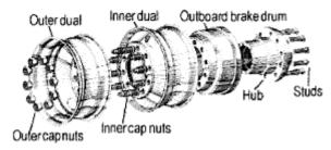
For dual wheels, this mounting system uses inner and outer cap nuts so that each wheel is tightened individually. For a front or single-rear wheel, a single cap nut is used. Right-hand and left-hand bolts and nuts are required. Wheels of this type can be identified by the spherical countersink surface around the individual bolt holes.
